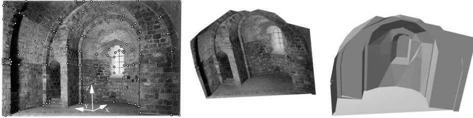
Fig. 6. Top: Indoor scene with 114 identified points. Bottom: Reconstruction obtained from these points and 39 known planes, shown with and without texture.
