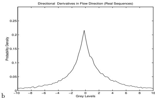
Fig. 1.: Histogram of the residues in Equation (1), using the affine flow approximation, computed from real images. The unknown flow parameters are replaced by a good estimate (computed off-line, allowing big computation resource). The tails are important : The variance is 39. This histogram was produced using 34000 measures and 500 bins. The residue is the sum of the noise terms ( $e_1$ ), ( $e_2$ ) and ( $e_3$ ), and a term due to the error in the estimate.
