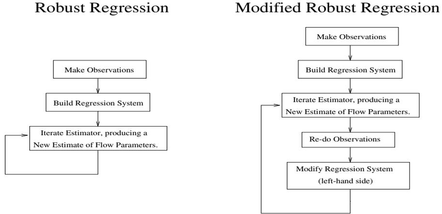
Fig. 2.: Block Diagram of the Robust Estimators : The left diagram corresponds to making one observation per image. In the right diagram, the observations are replaced at each iteration.
