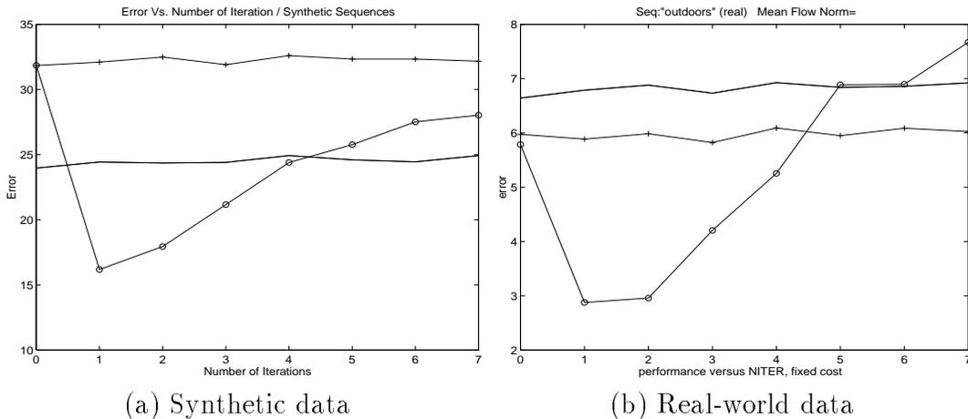
Figure 6: Empirical squared error of the estimator vs. number of iterations, for “Isotropic” (plain curve), “Anisotropic” (+) and “Anisotropic-M” (o) methods.
