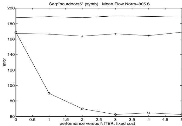
Figure 7: Empirical squared error of the estimator vs. number of iterations, for “Isotropic” (plain curve), “Anisotropic” (+) and “Anisotropic-M” (o) methods (All other conditions are equal). Number of observations is constant.
