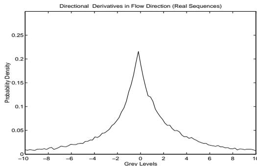
Figure 2: Histogram of the residues in equation (4), using the affine flow approximation, computed from real images. The unknown flow parameters are replaced by a good estimate; thus there is an extra error term. The tails are important : The variance is 39. This histogram was produced using 34000 measures and 500 bins.
