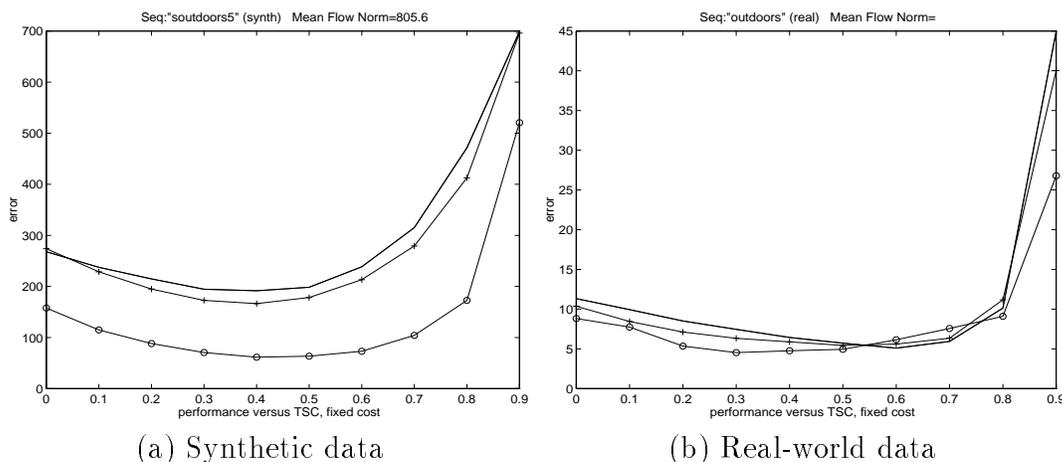
Figure 5: Empirical squared error of the estimator vs. time-smoothing coefficient, for “Isotropic” (plain curve), “Anisotropic” (+) and “Anisotropic-M” (o) methods.
